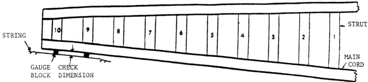
Record Distortion In Main Chord between Cross Struts
