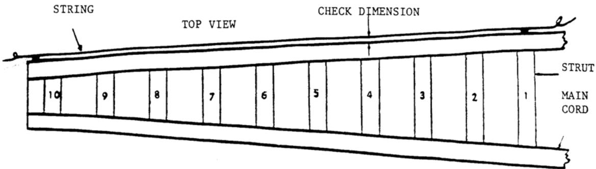
1. Place gauge blocks on the outside of the main chords, one on each end of the jib, and pull Maximum Check Dimension the string tightly over them.
