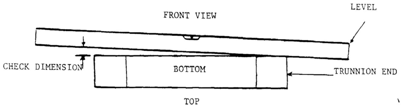
1. With the jib bottom up, level the front end of the jib.
